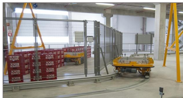
Monorail conveyor (on floor)
